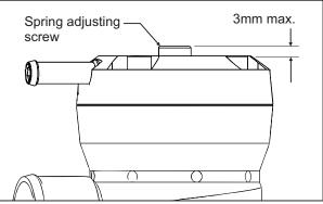
NOTE: On some cars, access to the adjustment screw is blocked by the ignition coil pack. In this case, it is easiest to loosen the valve mounting bolts 1 turn, then rotate the valve upwards just enough to make spring adjustments, then rotate the valve back down and re-tighten the mounting bolts.
